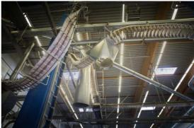
UTR conveyor chains have now cleared a path to reorganizing material flow and production processes at Druckhaus Wittich Föhren. This was an important step towards automating currently manual production stages.
