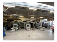
Having four compensating stackers lined up in a row now makes it possible to distribute several productions between them in whichever way is optimal for bundle formation.
